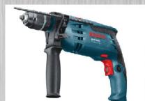
701W Impact Drill, Keyless Chuck, Carry Case, 0-3,000rpm, 16mm drilling capacity in concrete.VSR, Soft grip, Compact size 1.7kg, Carry case. Suitable for Trade.
